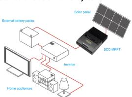
Combined MPPT technology and DSP controller, SCC-MPPT will convert best voltage to charge battery based on varied temperature. Compared to traditional solar charge controllers, it allows your solar panels to operate at their optimum power output voltage, providing higher efficiency up to 98% with lower power loss.
