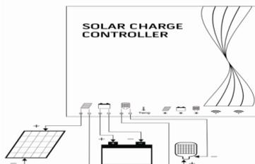
Connection sequence: Please connect the storage battery first, then connect the load, last is the solar panel. Pay attention to the “+” and “-” in case of reverse connection.
